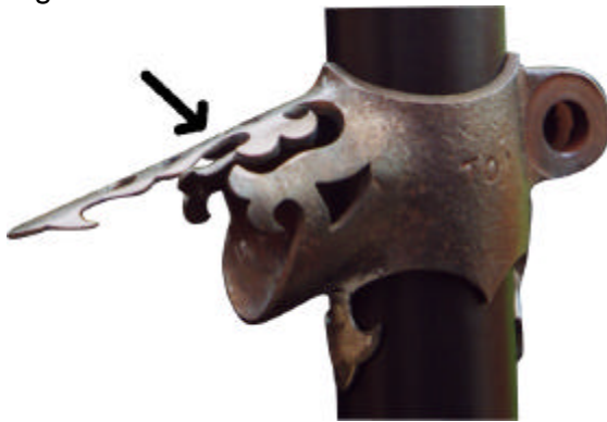
Magnum Opus casting showing the point where the extension was welded on.
